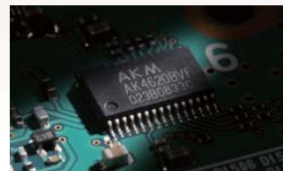
<AD/DA converter> AK4620B ADC Signal/(Noise+Distortion) : 100dB ADC Dynamic range, S/N : 113dB DAC Signal/(Noise+Distortion) : 97dB DAC Dynamic range, S/N : 115dB
