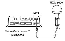
(Example: Connect to the MarineCommander<sup>™</sup>) Prior to any operation, it is important to make sure that all connections are made accurately. All connections should be made only by certified persons.
