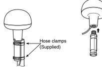
The supplied extension pipe is to be inserted firmly into the base of the GPS receiver and screwed in a clockwise direction.
